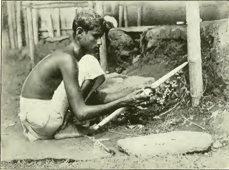
FIG. 1.—RUBBING DOWN THE INNER SURFACE OF A CHANK WORKING SECTION, DINAJPUR, BENGAL.
