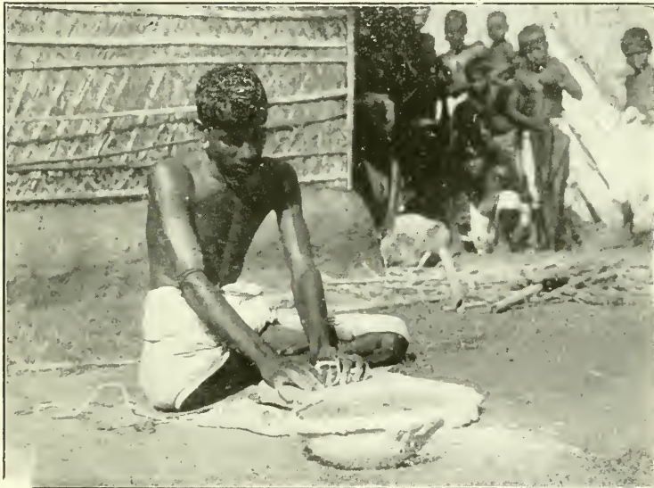
FIG. 2.—FORMING A SIMPLE RIDGE PATTERN BY RUBBING DOWN THE SECTIONS ON A STONE, RANGPUR, BENGAL.
